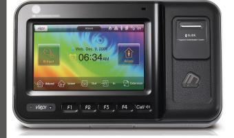
AC 6000 is a high-end state of the art access & time control recording fingerprint terminal. It has onboard Color camera to record the images of users as they transact (accepted and rejected transactions), USB I/F and TCP/IP interface. It has Face detection as special feature and stores
